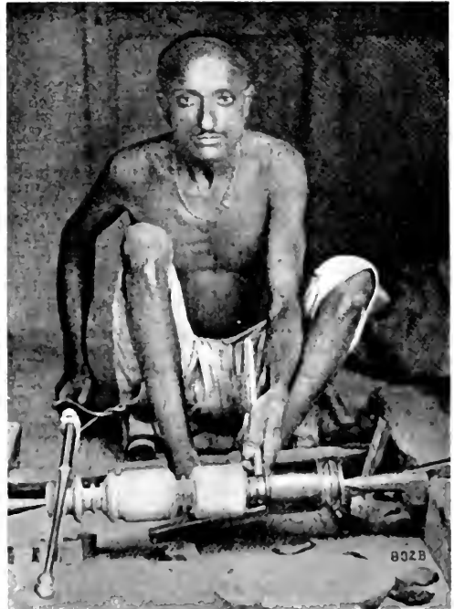
Fig. 9. AN ORIENTAL BOW LATHE. The bow or driving device is held in the right hand and the cutting tool in the left. Note the long centers upon which the work is mounted.
